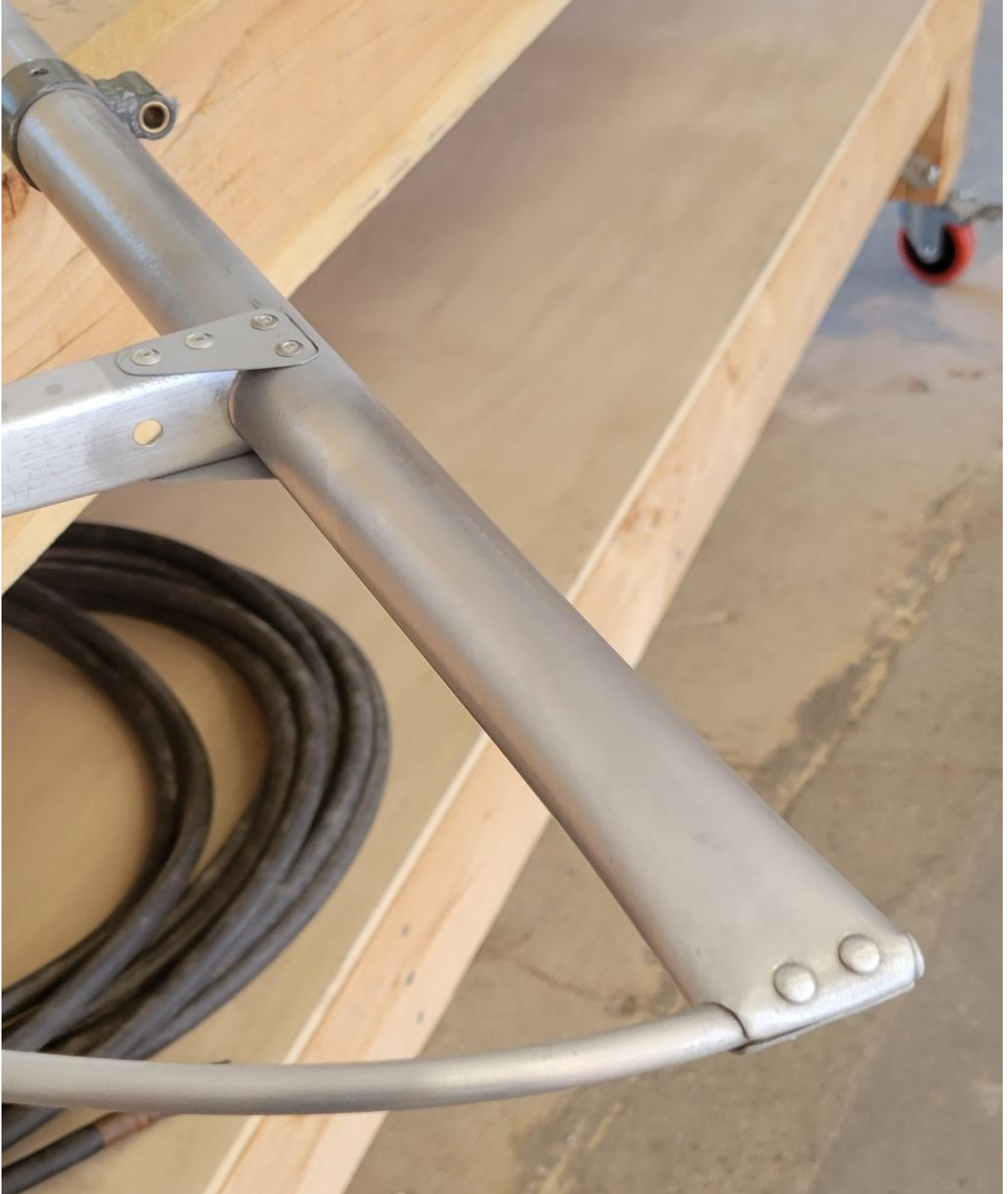
A finished spar tip, courtesy of builder Glenn Gordon.
